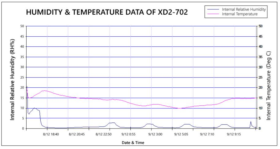
Test Conditions: Observe the humidity change in an unloaded XD2-702-01 for 19 hours. Test Result: The humidity level in XD2-702-01 is maintained at an average of 0.9% after the RH levels become stable below 5% to satisfy IPC/JEDEC (both 033 and 020) standards.
