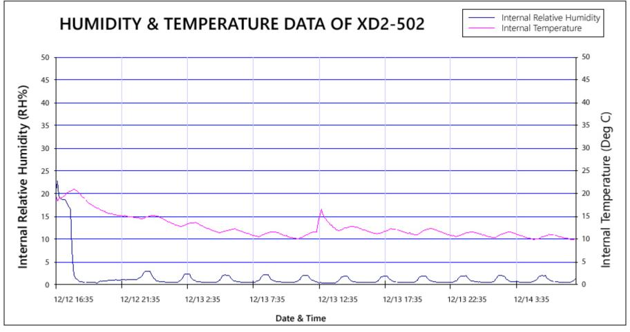
Test Conditions: Observe the humidity change in an unloaded XD2-502-01 for 72 hours. Test Result: The humidity level in XD2-502-01 is maintained at an average of 1% after the RH levels become stable below 5% to satisfy the IPC/JEDEC (both 033 and 020) standards.
