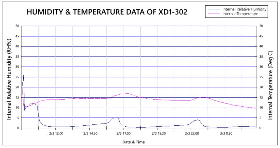
Test Conditions: Observe the humidity change in an unloaded XD1-302-01 for 24 hours.
