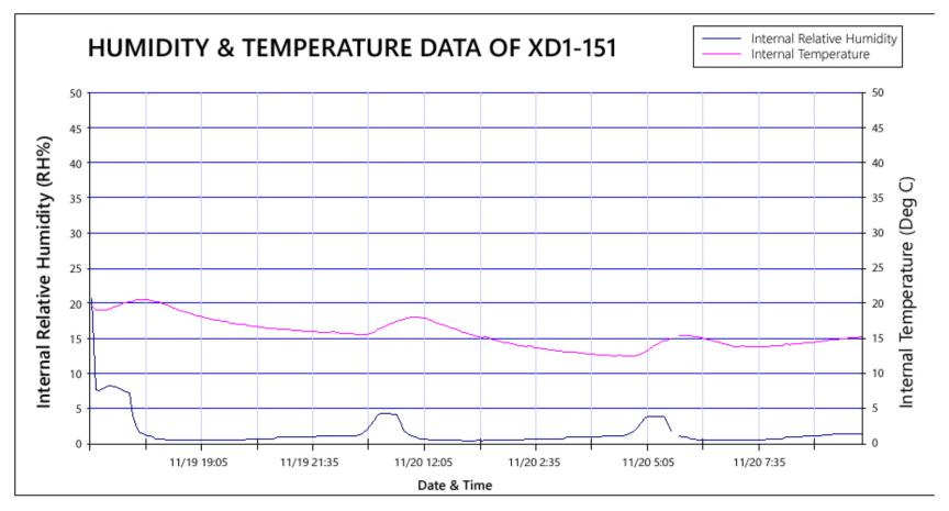
Test Conditions: Observe the humidity change in an unloaded XD1-151-02 for 18 hours.
